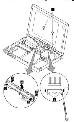
The status indicator has three latches on its rear and two in its front. in step 3, do as follows:
